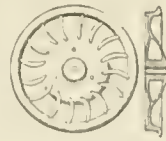
Washburn Car-wheel; side elevation and diametric section.
